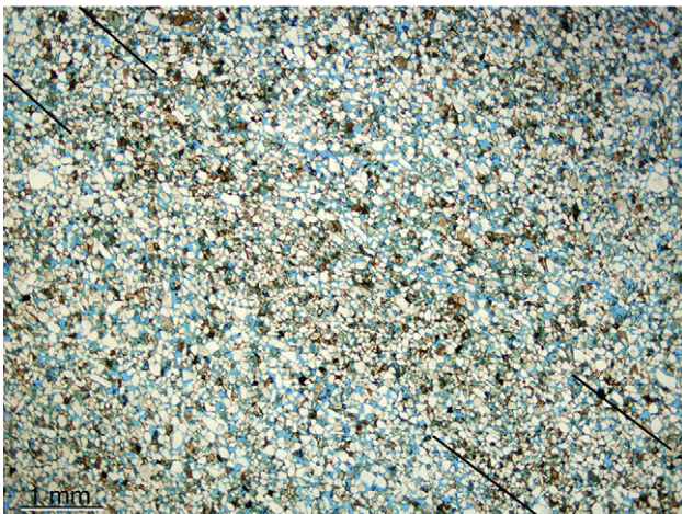
Fig. 7. Typical disaggregation deformation band of the Dewey Bridge Mbr., running diagonally across the picture.
